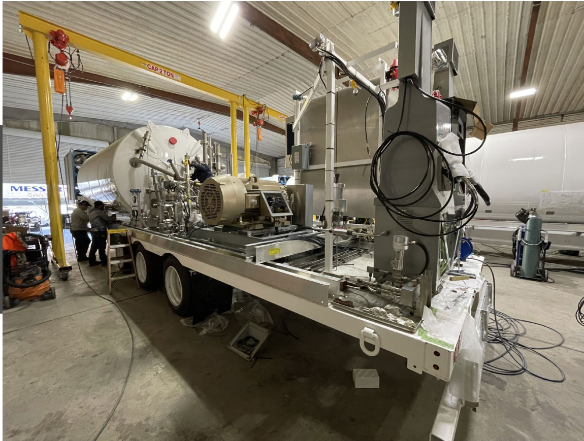
Mobile Hydrogen Refueler to be delivered to North Base
